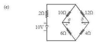
Find the Thevenin and Norton equivalent circuits with respect to the terminals a, b of this network.
